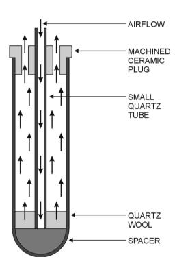
Air percolates through the quartz wool, oxidising any pollutants and rendering them harmless and unable to penetrate the quartz sheath of the thermometer.
